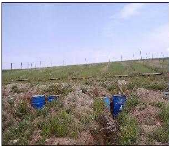
Fig 1: The tanks for collecting runoff
